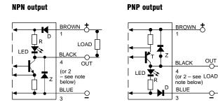
NOTE: in case of combined load, i.e. resistive and capacitive, the maximum admissible capacity (C) is  $0.05\mu\text{F}$  for maximum output voltage and current.
