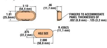
Material Flammability Rating Temperature Rating Polycarbonate 94V-2 -40°F (-40°C) to 239°F (115°C)
