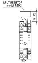
Input shunt resistor attached for current input
