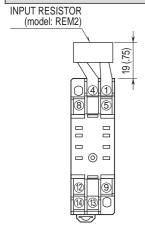
Input shunt resistor attached for current input.
