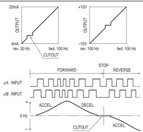
Forward Rotation: Phase A leads the Phase B by 90 degrees. Reverse Rotation: Phase A lags behind Phase B by 90 degrees.
