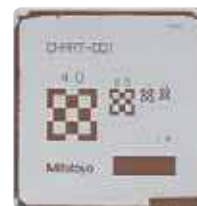
Calibration gage (02AQC310) - Gage for sharing the coordinates between the QVP and contact-type probe
