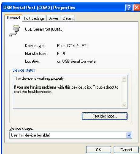
Figure 2.8 – Access COM Port Properties
