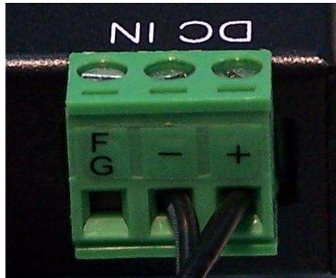
Figure 1 9V DC to 48V DC power input connector
