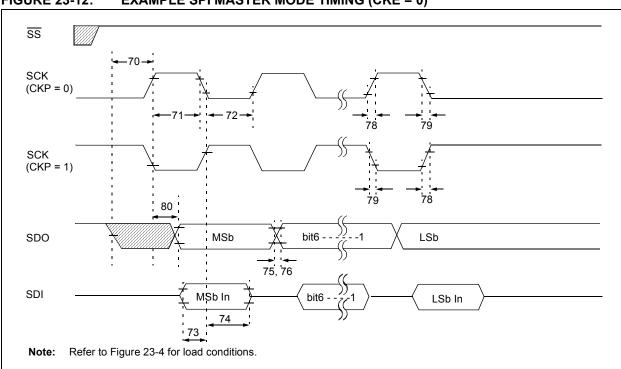
FIGURE 23-12: EXAMPLE SPI MASTER MODE TIMING (CKE = 0)
