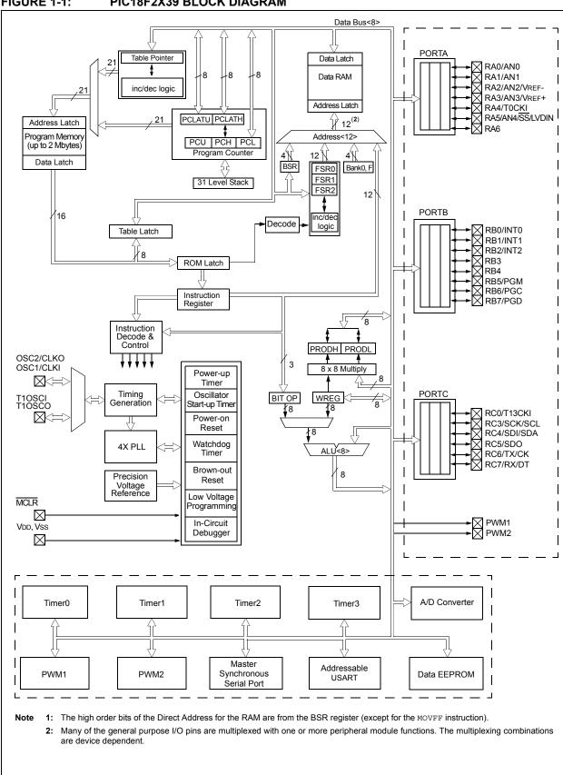
FIGURE 1-1: PIC18F2X39 BLOCK DIAGRAM
