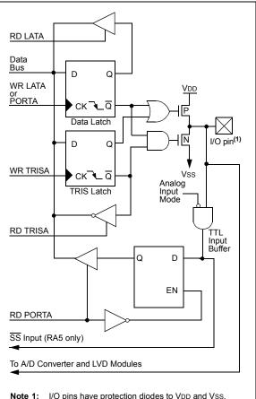
Note 1: I/O pins have protection diodes to VDD and Vss.
