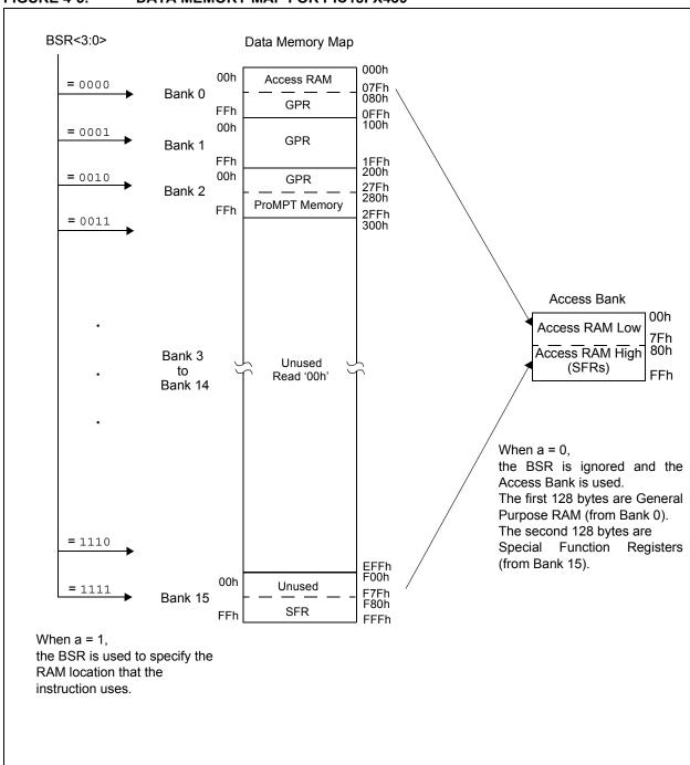
FIGURE 4-5: DATA MEMORY MAP FOR PIC18FX439
