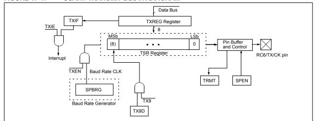
FIGURE 17-2: ASYNCHRONOUS TRANSMISSION
