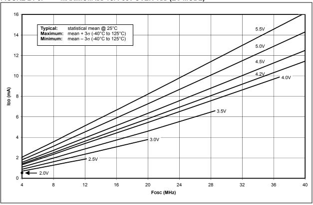
FIGURE 24-7: IPD vs. VDD, -40°C TO +125°C (SLEEP MODE, ALL PERIPHERALS DISABLED)
