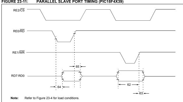
FIGURE 23-11: PARALLEL SLAVE PORT TIMING (PIC18F4X39)
