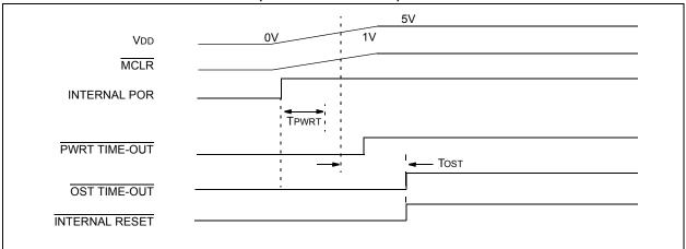
FIGURE 3-7: TIME-OUT SEQUENCE ON POR W/ PLL ENABLED (MCLR TIED TO VDD)
