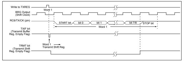
FIGURE 17-3: ASYNCHRONOUS TRANSMISSION (BACK TO BACK)
