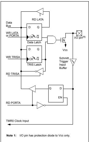
FIGURE 9-3: BLOCK DIAGRAM OF RA6 PIN
