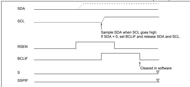
FIGURE 16-30: BUS COLLISION DURING REPEATED START CONDITION (CASE 2)
