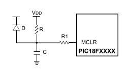
Note 1: External Power-on Reset circuit is required only if the VDD power-up slope is too slow. The diode D helps discharge the capacitor quickly when VDD powers down.
