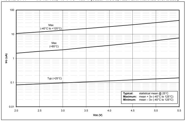
FIGURE 24-8: △IBOR vs. VDD OVER TEMPERATURE (BOR ENABLED, VBOR = 2.00 - 2.16V)
