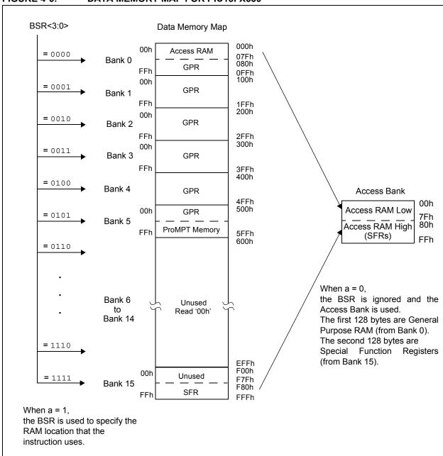
FIGURE 4-6: DATA MEMORY MAP FOR PIC18FX539
