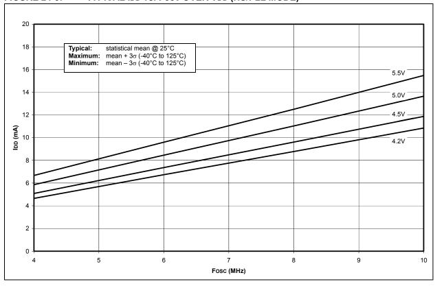
FIGURE 24-4: MAXIMUM IDD vs. Fosc OVER VDD (HS/PLL MODE)
