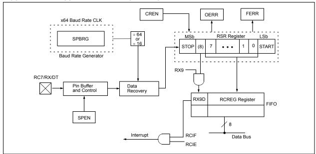
FIGURE 17-5: ASYNCHRONOUS RECEPTION
