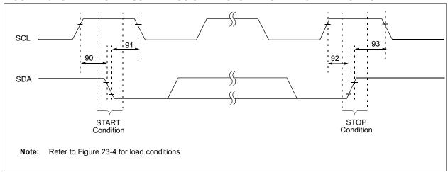
TABLE 23-17: MASTER SSP I<sup>2</sup>C BUS START/STOP BITS REQUIREMENTS
