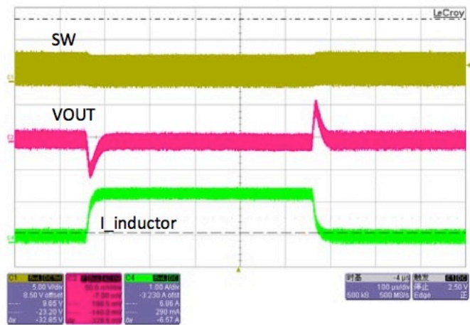
Load Transient V_{in}=3.6V , V_{out}=1.8V , I_{out}=0.2A/1.5A
