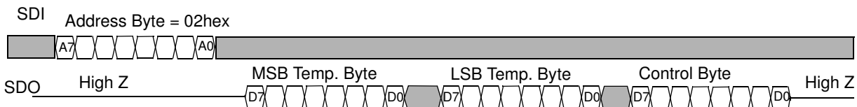
FIGURE 4-3: Serial Interface Timing Diagrams (CP=0).
