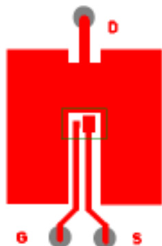
③ Surface mounted on 1 in. square Cu (still air).
