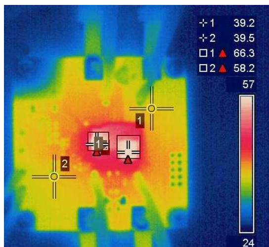
Figure 16: Thermal Image at V_{IN} = 12V , I_{OUT} = 8A (IR3871: 66^\circ C , Inductor: 58^\circ C , PCB: 40^\circ C )
