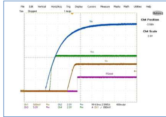
Figure 31: Start up at 12A Load, Ch 1 : V out , Ch 2 :V in , Ch 3 :P Good , Ch 4 :V cc
