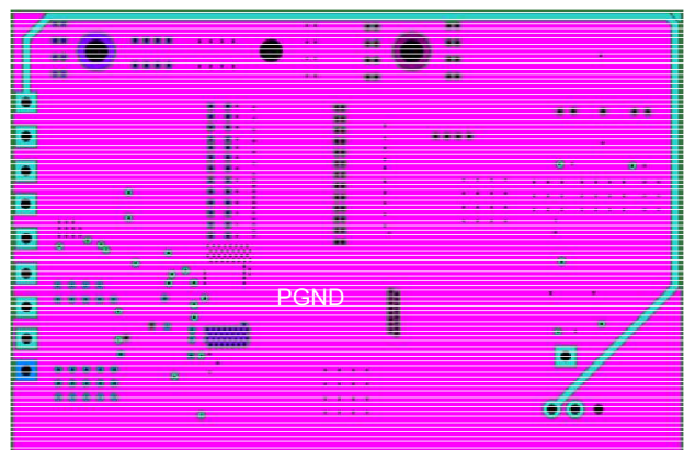
Figure 35f: IRDC1827 demoboard layout considerations – Mid Layer 4
