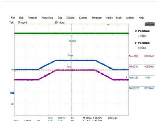
Figure 47: Voltage Margining using Vref pin Ch2-Vo, Ch3-Vref, Ch4-pGood
