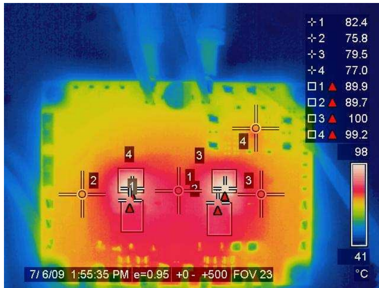
Fig. 16 Thermal Image: I_{out} = 60A , V_{IN} = 12V , with Internal VDD, V_{OUT} = 1.2V , T_A = 45^\circ C , f_{sw} = 500kHz , 200LFM, No Heatsink
