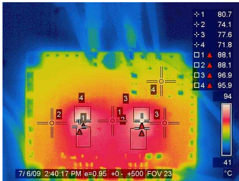
Fig. 17 Thermal Image: I_{out} = 60A , V_{IN} = 12V , V_{DD} = 6V , V_{OUT} = 1.2V , T_A = 45^\circ C , f_{sw} = 500kHz , 200LFM, No Heatsink
