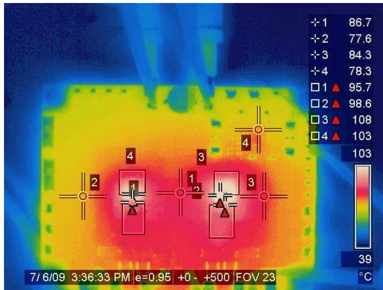
Fig. 24 Thermal Image: I_{out} = 30A per channel, V_{IN} = 12V , with Internal VDD, V_{OUT1} = 1.5V , V_{OUT2} = 2.5V , T_A = 45^\circ C , f_{sw} = 500kHz , 200LFM, No Heatsink
