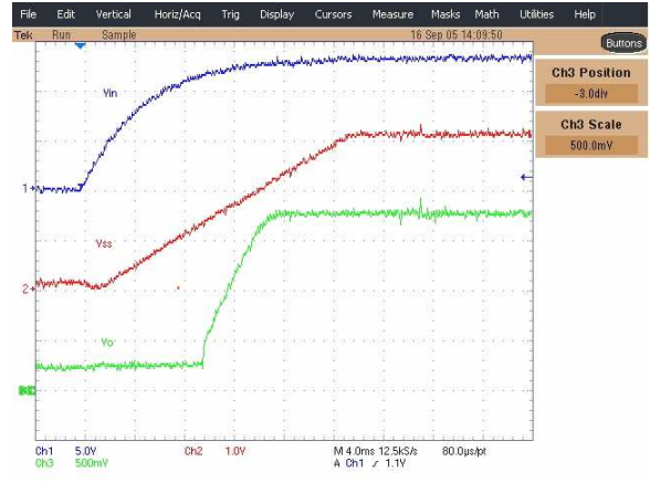
Fig.18: Pre-Bias Start up Ch 1 :V in , Ch 2 :V ss , Ch 3 :V o
