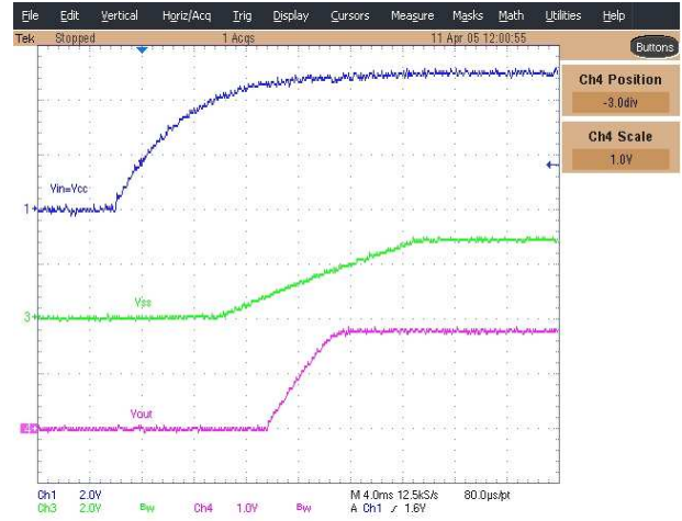
Figure 15 - Start up waveforms Ch1: Vin=Vcc, Ch3: Vss, Ch4: Vout
