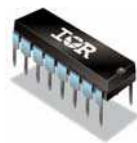
16-Lead PDIP IRS2168DPbF
