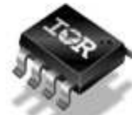
8-Lead SOIC IRS2301S
