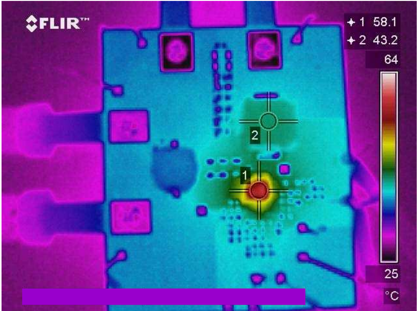
Fig. 17: Thermal Image at 8A load Test points 1 and 2 are IR3841W and inductor, respectively.
