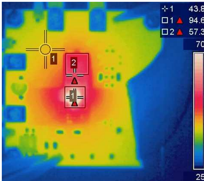
Fig. 17: Thermal Image (IR3475: 95°C, Inductor: 57°C, PCB: 44°C)
