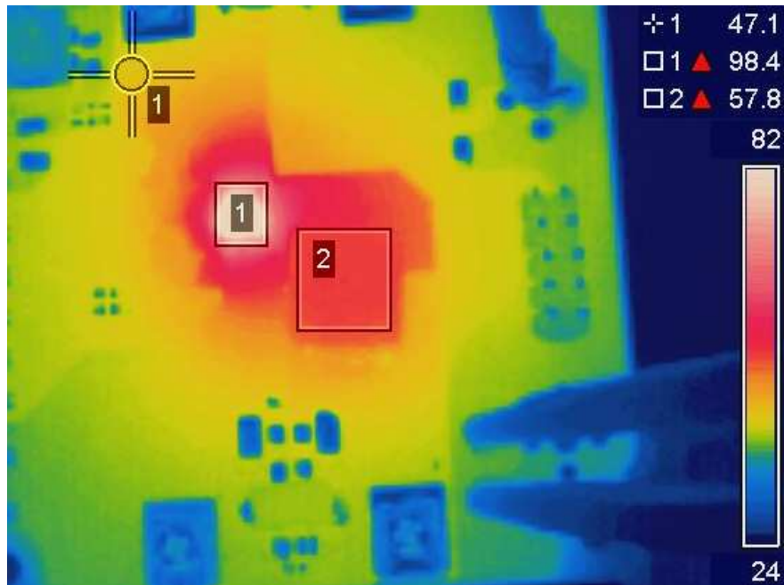
Fig. 17: Thermal Image (IR3476: 98°C, Inductor: 58°C, PCB: 47°C)
