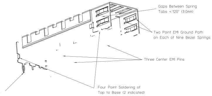
Eleven press-fit (compliant) pins for single sided use in .062+" (1.57+mm) PCB's with tin plated through holes.
