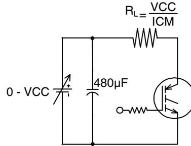
**Fig. 13b** - Pulsed Collector Current Test Circuit
