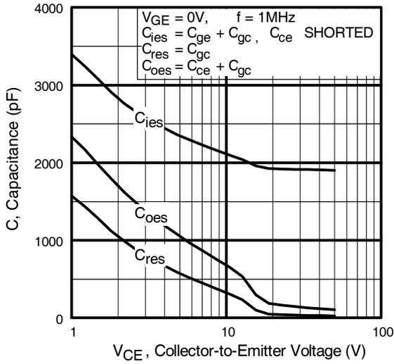
**Fig. 7** - Typical Capacitance vs. Collector-to-Emitter Voltage
