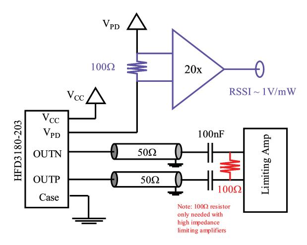
Optional RSSI implementation is shown in blue Optional  $100\Omega$  differential termination for high impedance limiting amplifiers is shown in red.
