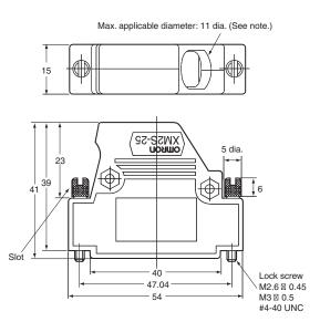
**Note:** The maximum applicable cable diameter is 9 dia if the cable clamp supplied is mounted facing the rear. Do not use a cable bushing in this case.
