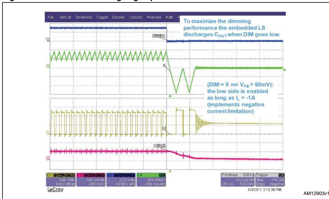
Figure 12. LED current falling edge operation
