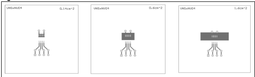
Figure 37. SO-8 PC board (1)
