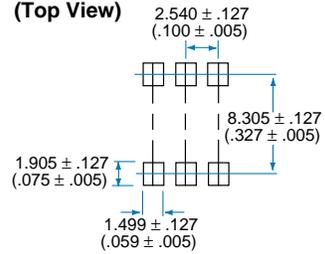
Tape and Reel Packaging for 6 Pin Surface Mount Package
