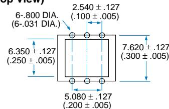
**6 Pin DIP Surface Mount ("S" Suffix)**
