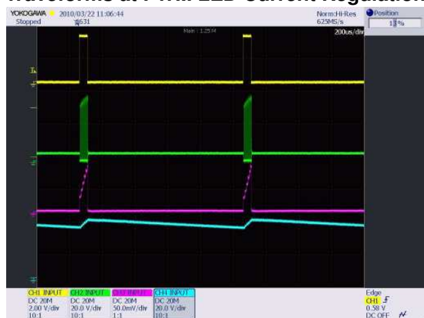
Ch 1 (yellow) – PWM signal at 1 kHz 5% duty cycle Ch 2 (green) – SW node voltage, Ch 3 (red) – LED Current. Ch 4 (blue) - V_{OUT}
