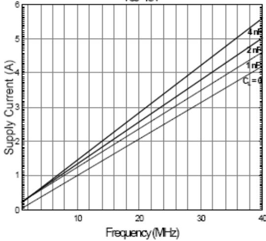
Fig. 7 Supply Current vs. Load Capacitance
