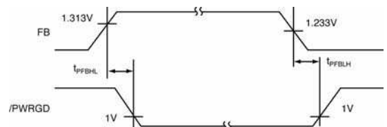
Figure 4. MIC2587/87R-2 FB to /PWRGD Timing
