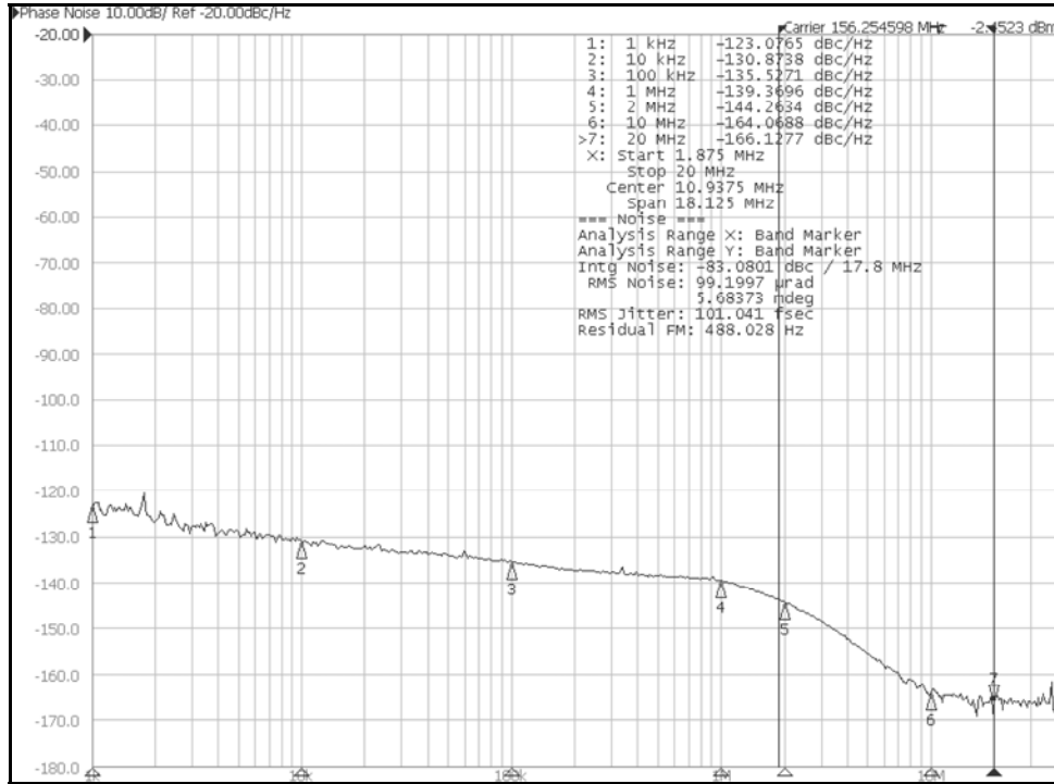
Phase Noise Plot: 156.25MHz, 1.875MHz – 20MHz 101fS
