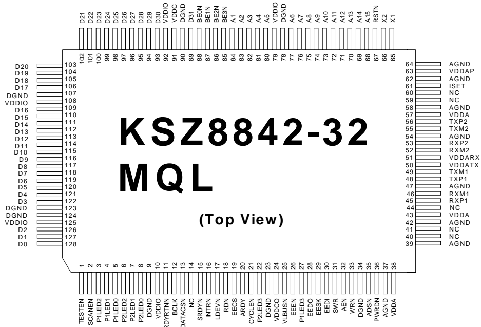
Figure 5. Standard – KSZ8842-32 MQL 128-Pin PQFP (Top View)
