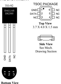
**NOTE:** The leads of TO-92 packages on tapeand-reel are formed to approximately 100 mil (2.54 mm) spacing. For details see the *Package Information* section.
