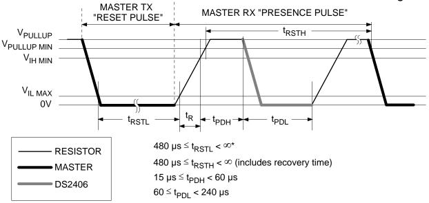
\* In order not to mask interrupt signaling by other devices on the 1-Wire bus,  $t_{RSTL} + t_R$  should always be less than 960 $\mu$ s. In a parasitically powered environment  $t_{RSTL}$  should be limited to maximum 5ms. Otherwise the DS2406 may perform a power-on reset.
