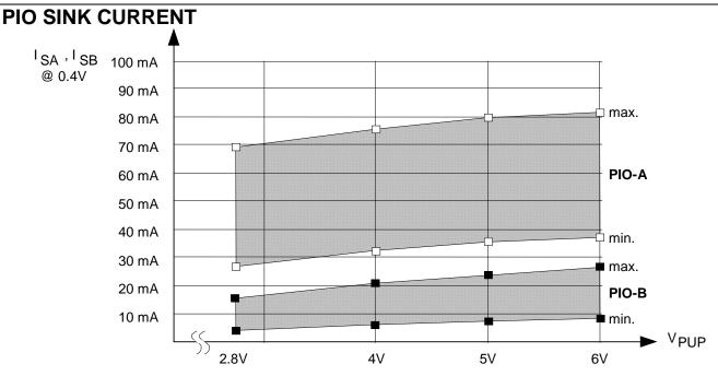
**NOTE:** The sink current is production-tested at  $V_{PUP} = 2.8V$ ; the specification for  $V_{PUP}$  of 4V, 5V and 6V is guaranteed by design.
