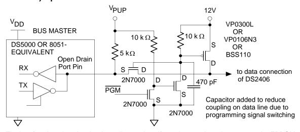
The interface is reduced to the  $5k\Omega$  pull-up resistor if one does not intend to program the EPROM cells.
