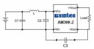
**Note A:** An external filter capacitor is required if the module has to meet EN61000-4-4 and EN61000-4-5. The filter capacitor Aimtec suggests: 1000uF, 100V.
