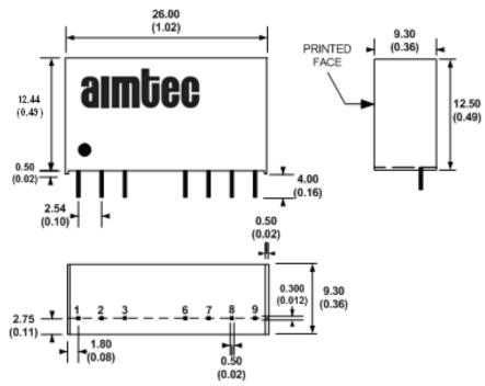
All dimensions are in millimeters (inches) Pin diameter: 1.0  $\pm$ 0.05 ( 0.04  $\pm$ 0.002 ) Pin pitch tolerance:  $\pm$ 0.35 (  $\pm$ 0.014 ) Case Tolerance:  $\pm$ 0.5 (  $\pm$ 0.02 )
