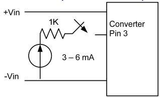
The voltage could be applied trough a limiting resistor. The converter is turned on the external switching circuit is open.
