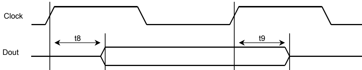
Figure 18-5. To/From High-Z Delay Definitions (Rising Clock Edge)
