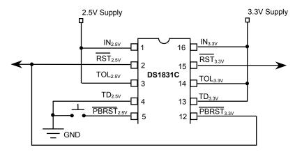
NOTE: The  $\overline{\text{RST}}_{2.5}$  volt output is connected to the  $\text{IN}_{3.3\text{V}}$  via a  $100\text{k}\Omega$  resistor in the pushbutton input and therefore does not require a pull-up resistor (an addition pull up can be used to accelerate responses.) If an external pull-up is used in this example it must be connected to the 3.3V power supply.
