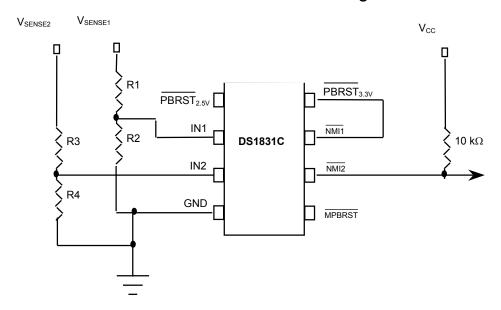
Example:  $V_{SENSE1} = 11.50 \text{ volts trip point}$   $V_{SENSE1} = \frac{R1 + R2}{R2}$  X 1.25V
