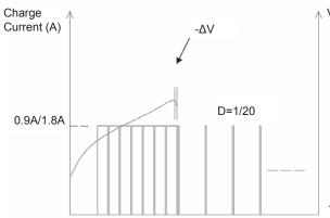
Voltage (V) This charger can charge between 8 and 15 NiMH or NiCd cells connected in series and will detect and provide the correct output voltage and current to suit.
