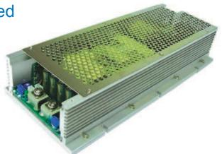
The PSL400BP Series has been designed as a ruggedized power supply housed in a robust extruded aluminium chassis designed for use in industrial or other types of equipment where cooling fans are undesirable and convection airflow is not available. Units can be mounted in a sealed box providing that the external heat sinking is adequate to maintain the baseplate at a temperature below 85° C.
