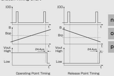
This Hall IC's output is held as internal data just before the internal circuit turns OFF (IDD OFF). And after 24.4  $\,\mu$ s, the output changes. Note) 24.4  $\mu$ s in figures is typical value
