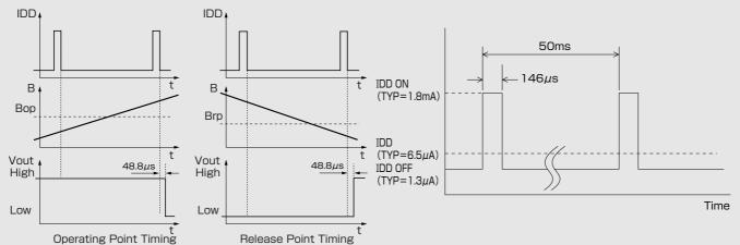
This Hall IC's output is held as internal data just before the internal circuit turns OFF (IDD OFF). And after 48.8  $\,\mu$ s, the output changes.
