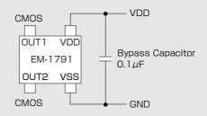
OUT1 responds to the positive flux from the south pole(Bop1,Brp1),OUT2 to the negative flux from the north pole(Bop2,Brp2) .
