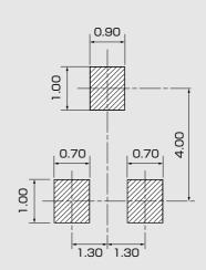
Note1) The sensor center is located within the  $\phi$ 0.3mm circle. Note2) The metal portions on the package side (support lead) are connected to the internal circuits. The support lead should be isolate from the external circuit and the other support lead.
