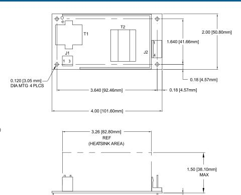
0.10 [2.54mm]MAX LEAD PROTRUSION
